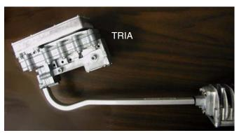
TRIA rotated for vertical polarization
